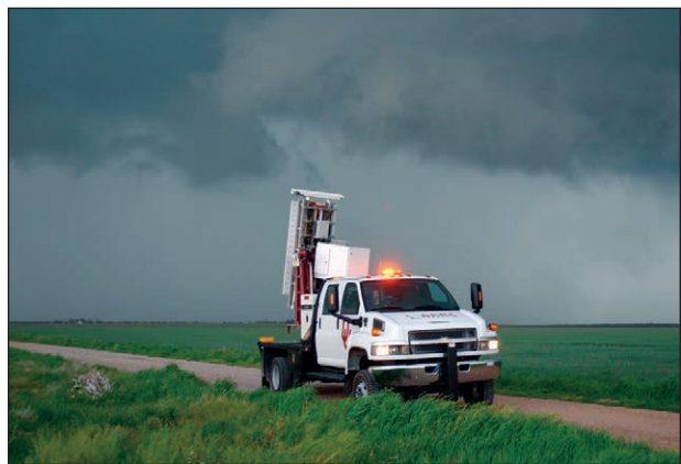
Fig. 3. A photograph of the atmospheric imaging radar (AIR) truck that was designed, built, and tested at the University of Oklahoma.
