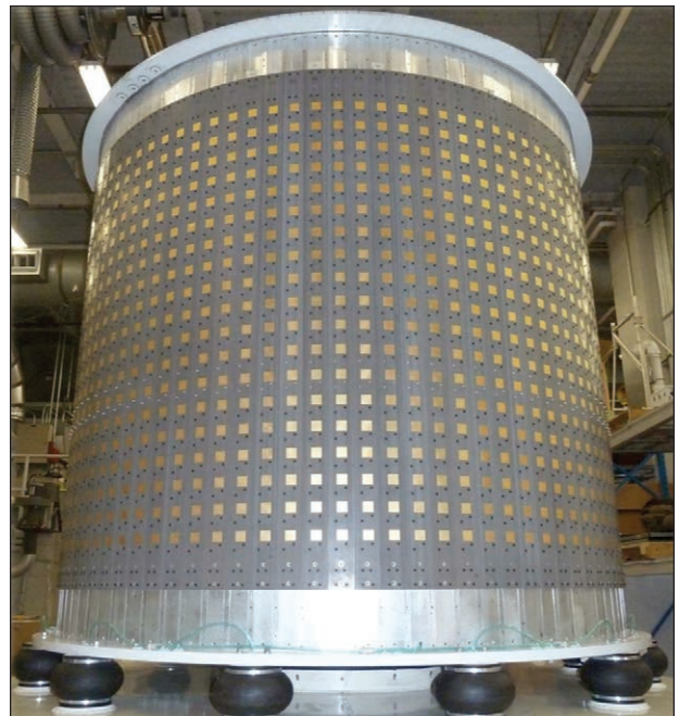
Fig. 5. Prototype phased array radar on a conformal cylinder. The size of the array is 1 m tall and 2 m in diameter and operates in a band near 3 GHz.
