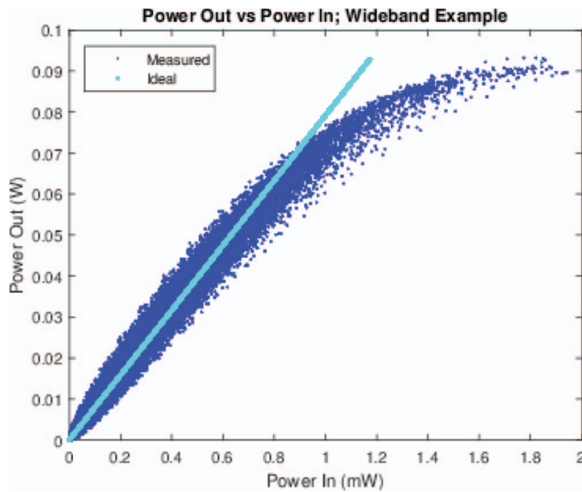
Fig. 3. Example of power out versus power in of measured wideband and ideal amplified signals.
