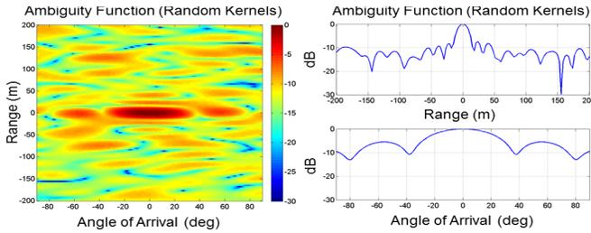
Fig. 3. A plot of the ambiguity surface of  $\mathbf{Y}$  centered on  $\tau_0$  is shown on the left with cuts through range ( $\psi = 0$ ) and angle ( $\tau = \tau_0$ ) shown to the right.
