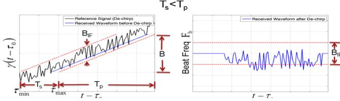
Fig. 2. An example of a uniformly random de-chirp, its frequency "hops" plotted vs. time and the results of de-chirping on a typical receive pulse, its beat frequencies plotted against time. Here  $T_s < T_p$ , so that de-chirp will vary over  $B_{IF}$  the implied bandwidth of range swath at any given moment
