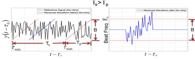
Fig. 1. An example of a uniformly random hopping de-chirp. Reference signal "hops" are shown vs. time, as well as the beat frequency time profile that results from the de-chirping process. Here  $T_s > T_p$ , so that the beat frequency will vary over  $B$  the bandwidth of the received signal
