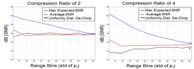
Fig. 4. A plot of SNR vs. the standard deviation of a Gaussian distributed target range measured in range bins for both a 2:1 and 4:1 compression (one range bin = 15m). Shown are the maximum expected SNR from the designed de-chirp plus the average SNR and SNR given a uniformly random de-chirp for a signal that would be 20dB SNR with no compression.
